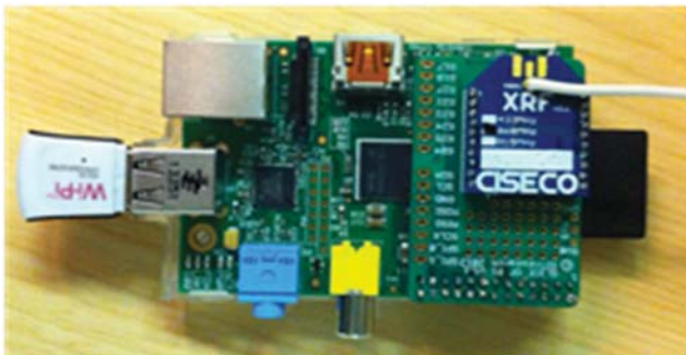
FIGURE 2. DTN Pi with 801.11 adapter and XRF receiver for wireless sensors.
