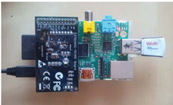
FIGURE 11. MODiToNeS Raspberry Pi B with a Xtrinsic sensor board and a WiPi wireless adapter.
