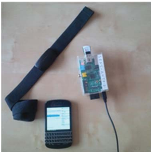
FIGURE 12. MODiToNeS Raspberry Pi with Suunto and WiPi USB module, Garmin heartrate sensor and a smartphone displaying readings.
