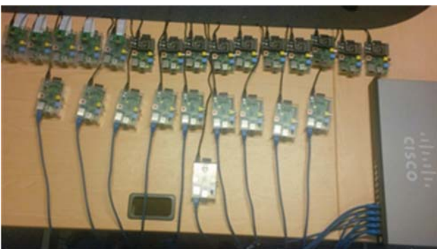
FIGURE 3. A hierarchical architecture Raspberry Pi sensor network example.
