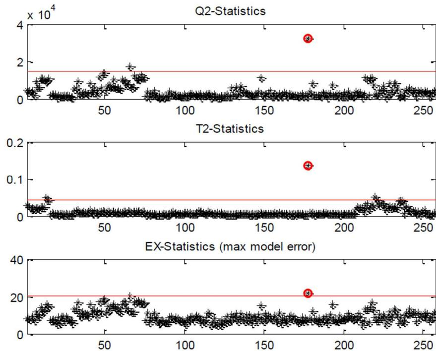
**Figure 8 - Statistical evaluation of welding traces to detect unusual shapes – Harms & Wende Demonstrator**
