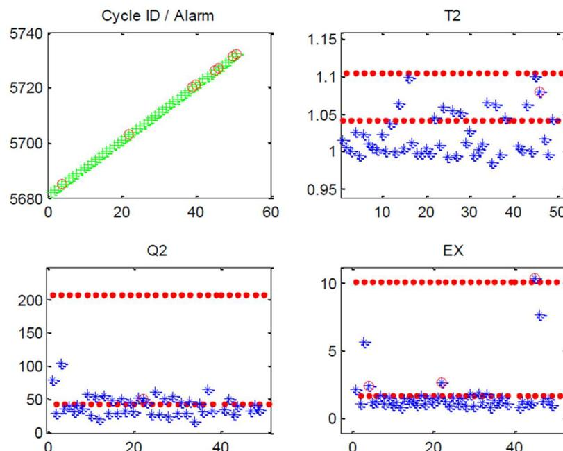
**Figure 7 - Statistical evaluation of traces to detect faulty movements – IEF Werner Demonstrator**
